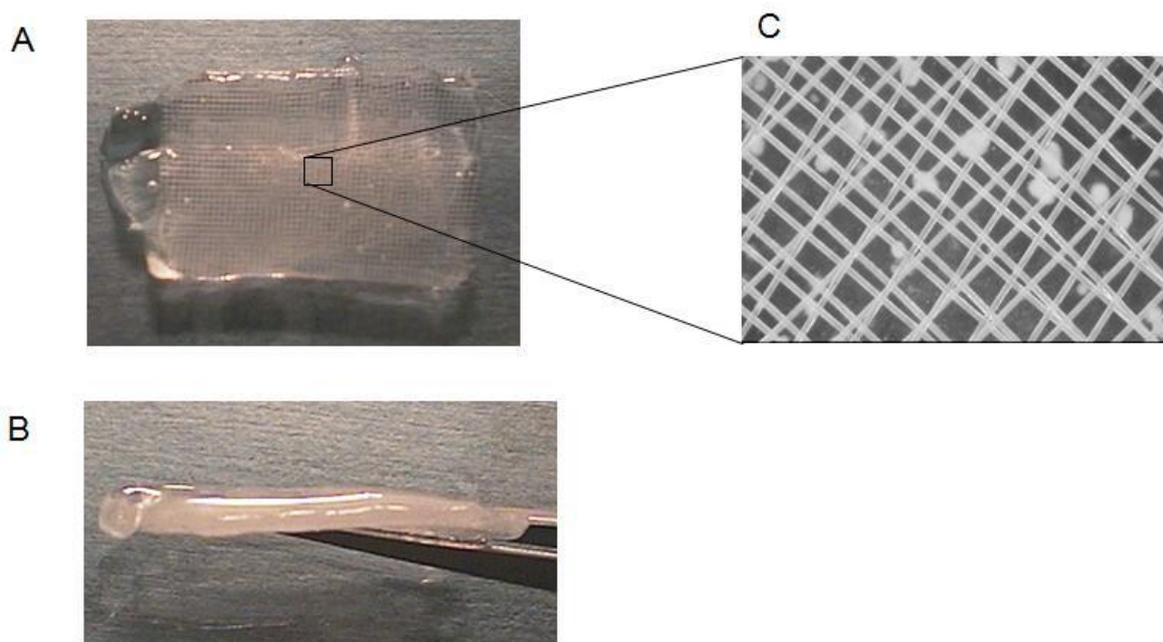
**Figure 2** A: A top-down view of mesh-reinforced PVA macro-encapsulated islets (PVA MEIs). B: A side view of PVA MEIs picked by tweezers. C: A microscopic view of PVA MEIs. Islets (round-shaped things) are entrapped in PVA gel between meshes.
