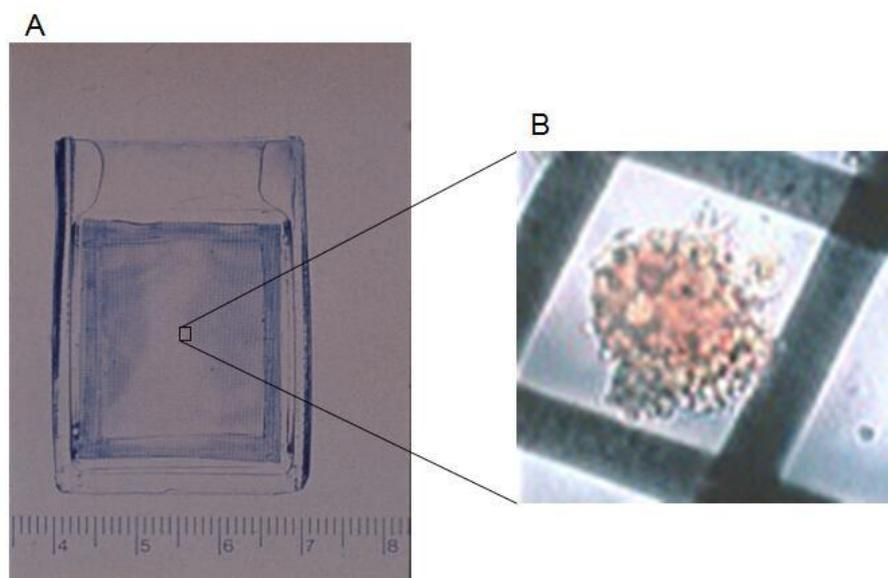
**Figure 1** A: A macroscopic view of a mesh-reinforced PVA bag (MRPB). B: A microscopic view of MRPB. An islet is trapped between mesh fibers.
